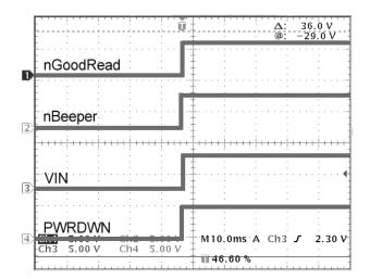
Figure 21. Power First Applied of TTL Version (Vin= 5V)
